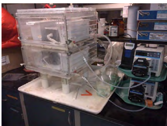
Figure 2. Prototype ammonia recovery system using gas-permeable modules (duplicate tests). One chamber circulated acid solution and the other circulated just water.
