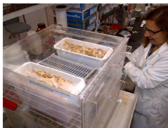
Figure 2. Prototype ammonia recovery system using gas-permeable modules (duplicate tests). One chamber circulated acid solution and the other circulated just water.
