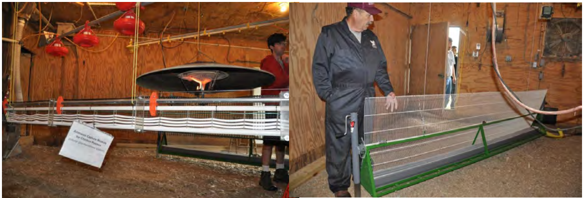
Figure 3. Pilot ammonia recovery systems installed in a chicken barn at UMES Poultry Research Facility. At left is a recovery module that uses tubular gas-permeable membranes. At right is a recovery module that uses flat as-permeable membranes.
