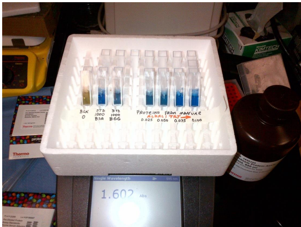
Figure 3. Extraction of proteins from manure and protein determination using Bradford method.
