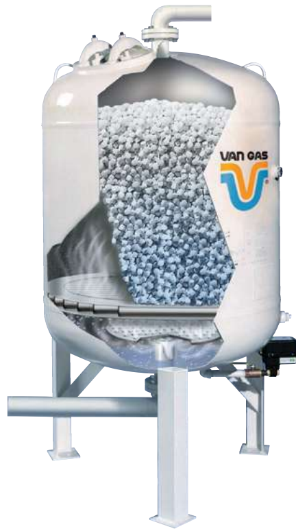
Figure 3. Example of a desiccator for water removal from the biogas: reactor filled with adsorbent material (zeolites).
